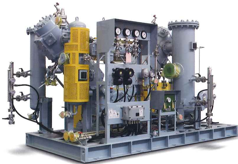
CH 4 Gas Model DYN6-2714G 2 Press. 2.2MPaG Req. Power 65kW
