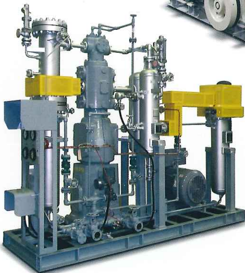
BF 3 Gas Model DNS6-1811B 3 G 2 Press. 3.9MPaG Req. Power 55kW
